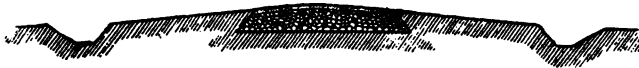
FIG. 24.—Section of macadam road with dirt tracks on either side. Shows ditches for surface drainage. (After a drawing in Yearbook, U. S. Dept. Agr., 1894, page 502.)
